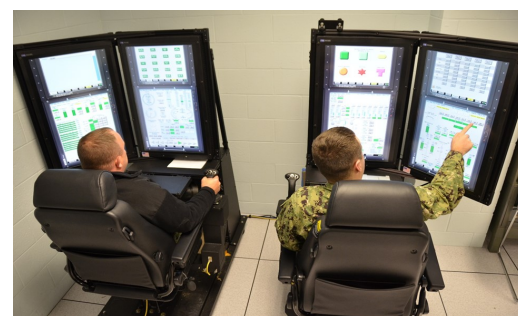
Sailors train on the Virginia Class Submarine Ship Control Operator Trainer VSCOT non-motion station
