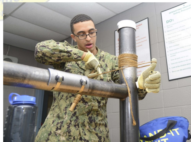
U.S. Navy Seaman Recruit Dylan Sanders practices the proper technique for making soft patch repairs using marlinspike during the Basic Submarine Damage Control course .
