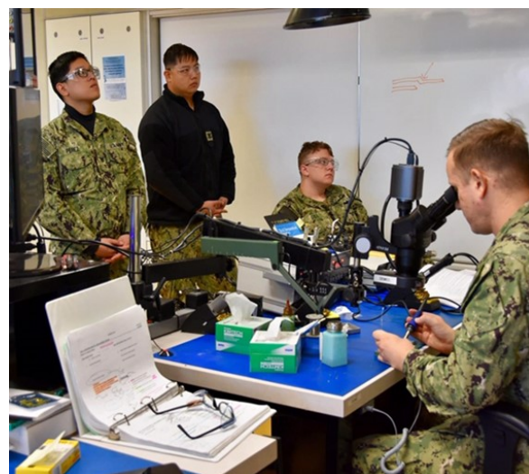
2M students preparing the CCA for a replacement eyelet during 2M Pipeline Course.
